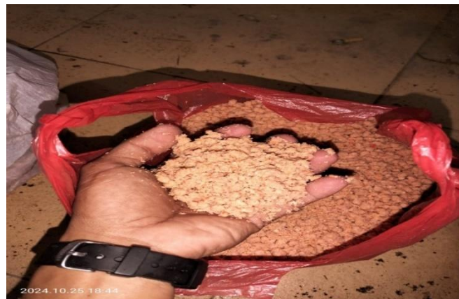
Figure 4. Results of grinding using a 7 mm sieve
