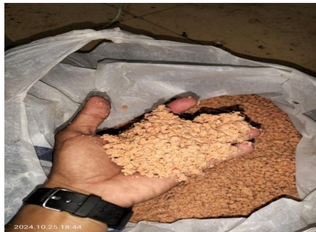
Figure 2. Results of grinding using a 5 mm sieve
