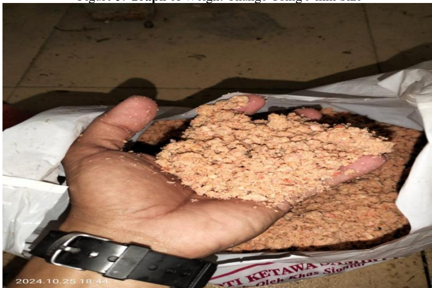
Figure 6. Results of grinding using a 9 mm sieve
